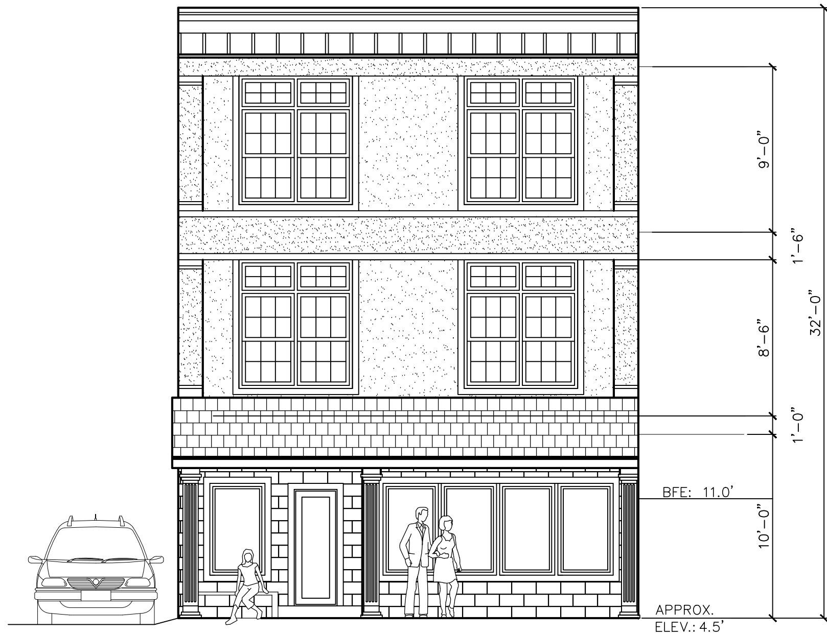
PROPOSED FRONT ELEVATION – 210 BAY AVE. SCALE: 3/16" –1'-0"
